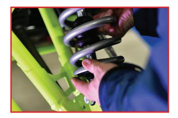
Remove OEM spring stack. Discard OEM springs. Keep and reuse OEM spring divider and OEM lower spring retainer. Take note of the spring retainer orientation, this will be placed back on the exact same way.
