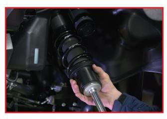
Install front new main spring and spring retainer.
