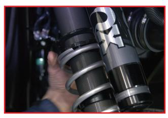
Move bump stop up 3 inches for removal of OEM lower spring retainer. Use flathead screwdriver.
