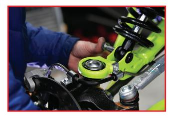
Set "zero Preload" by pressing down on A-arm and holding to fully extend internal bump stop spring. Rotate preload ring clockwise until spring stack contacts preload ring.
