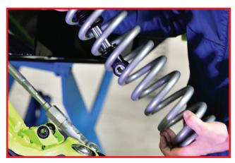
Install new Zbroz 6" front tender spring along with the spring retainer.
