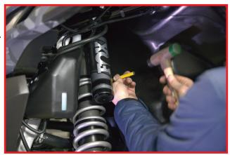
Rotate OEM preload rings counter clockwise all the way to top of threaded shock body. or until OEM spring stack is now loose.
