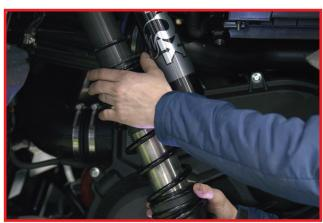
With a bright marker, mark your preload ring next to the reservoir. This is your "zero preload" point. From here you can set additional preload by tightening the crossover rings. \*Additional Preload may be needed depending on after-market accessories (bumper, cage, tire carrier, stereo system). 4-6 turns is a good starting point.
