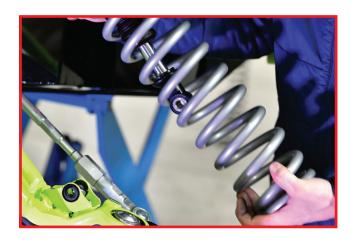
Loosen the OEM Crossover Rings while the springs are removed. Take a flathead screwdriver or punch, knock the top ring loose by tapping it counterclockwise.
