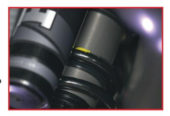
After you have set your preload, you will now set your crossover ring by measuring 3 1/4" from top of spring divider. Then tighten crossover ring screws. \*Additional Adjustments may be needed.
