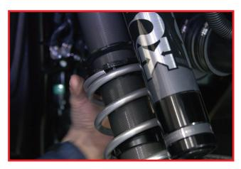
Pull the lower bumpstop up out of the way and push up on spring stack to remove OEM lower spring retainer.
