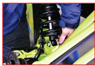
Set "zero Preload" by pressing down on trailing arm and holding to fully extend internal bump stop spring. Rotate preload ring clockwise until spring stack contacts preload ring.
