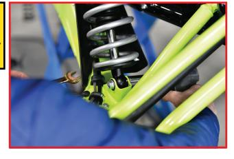
Loosen OEM upper preload ring from OEM lower preload ring. Use flathead screwdriver and hammer.
